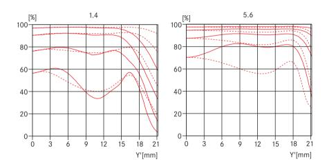
The MTF is indicated both at full stop and f/5.6 at long taking distances (infinity). Shown is the contrast in percentage for 5, 10, 20 and 40 lp/mm across the height of the 35 mm film format, for tangential (dotted line) and sagittal (solid line) structures, in white light. The 5 and 10 lp/mm will give an indication regarding the contrast ratio for large object structures. The 20 and 40 lp/mm records the resolution of finer and finest object structures.
