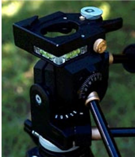
**Fig 1** Tripod head with double spirit levels
